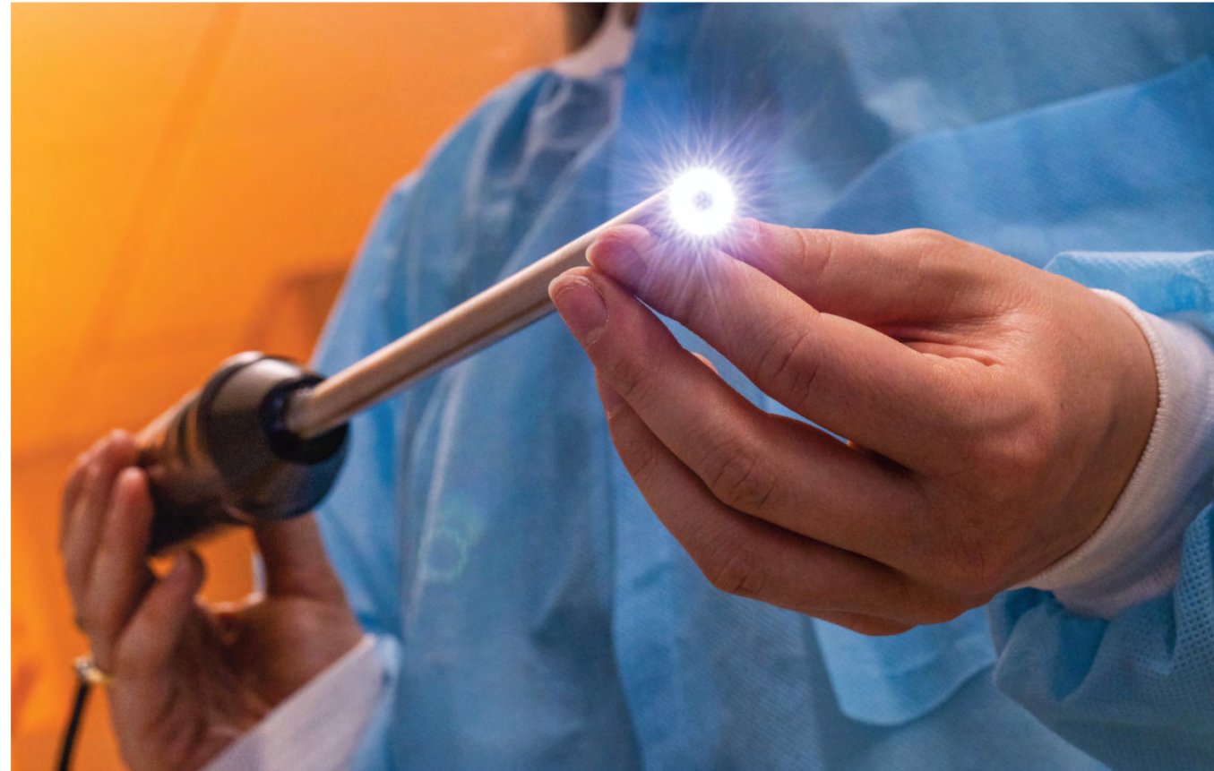
To illuminate the whole abdominal cavity without generating excess heat, a 5-millimeter ring of LED lights at the tip of the KeyScope device pulses in sync with the camera's frame rate.
